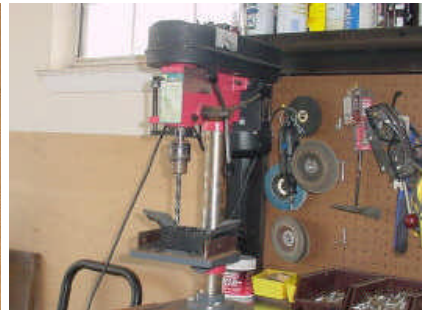
Drill 2- 25/64" holes in each mount
