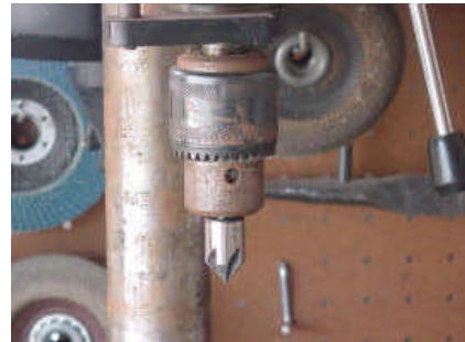
Counter sink the holes
