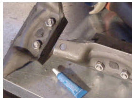
Using Loctite tighten nut until the bolt starts to spin plus an extra 1/4 to 1/2 turn.
