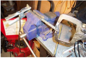
Grind a flat spot on the end of the rebar and tack a bolt to rebar
