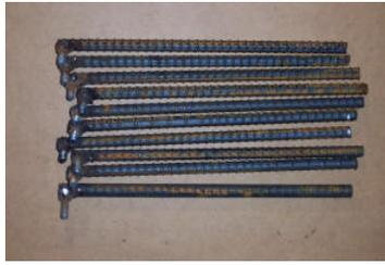
I used 5/16"x5/8" bolts and 3/8"x12" rebar
