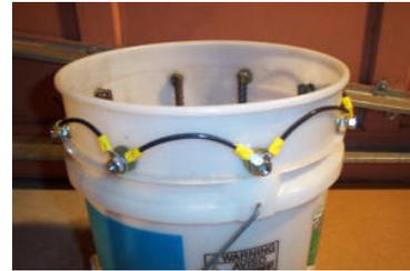
Flat washers on both sides of the plastic bucket and 10 gauge wire connected to each bar
